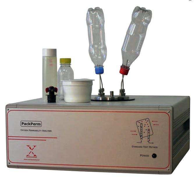
Oxygen Permeability tester. Packperm is a tester of permability to oxygen (02TR) for plastic bags, small containers, PET bottles, taps in bag-in-boxes, natural and synthetic crown or bottle corks and other products for packaging applications
